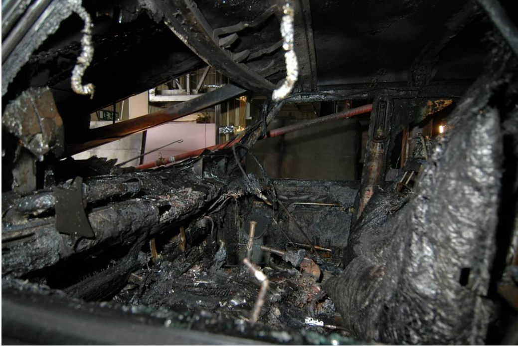
Figure 14 – Damage to interior of Land Rover (lower car)
