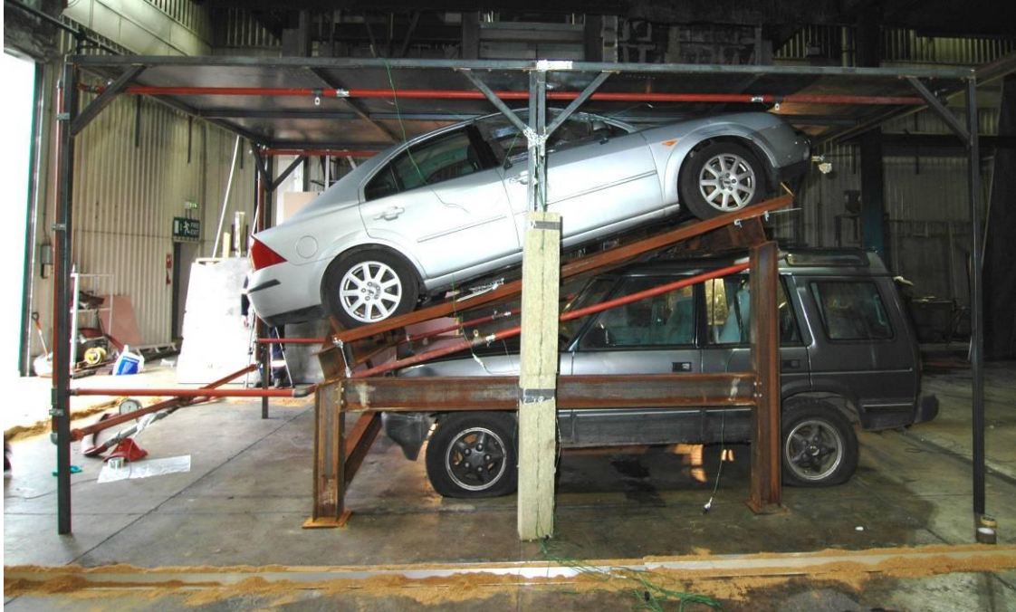
Figure 3 – Photograph showing test arrangement and sprinkler head positions (east side).
