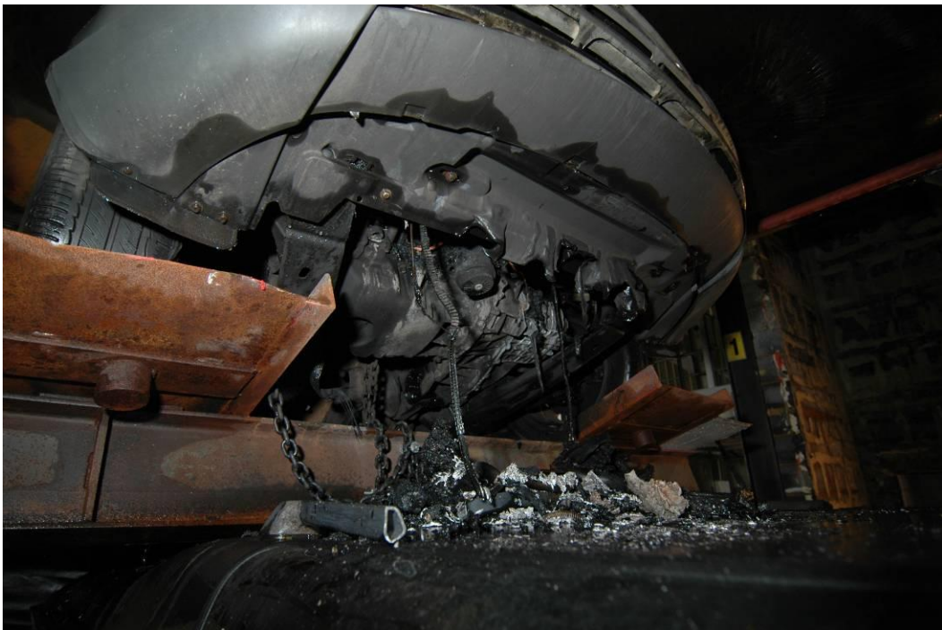
Figure 15 – Damage to underside and engine bay of Ford Mondeo (upper car)
