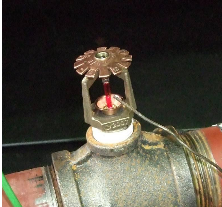
Figure 6 – Sprinkler head selected for testing
