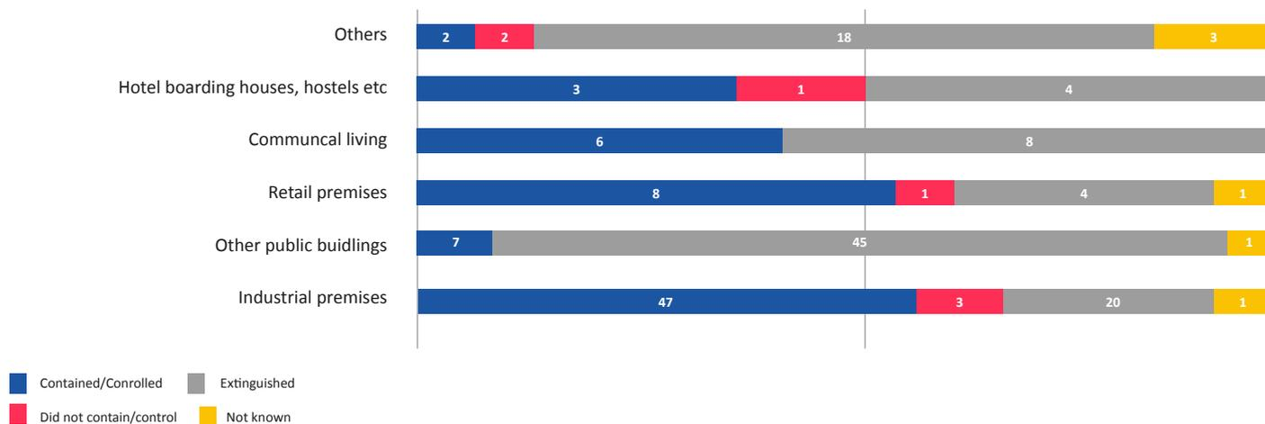
Figure 7 The effectiveness of the sprinklers system in containing the fire across the building type other buildings.
