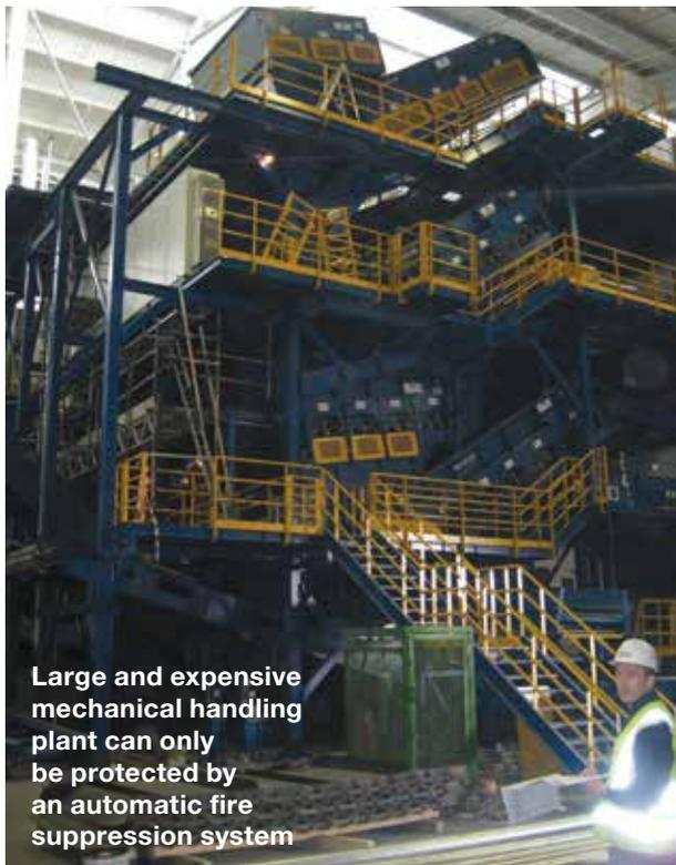
Large and expensive mechanical handling plant can only be protected by an automatic fire suppression system
