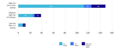
Figure 1. Number of sprinkler heads activated in purpose-built block of flats
