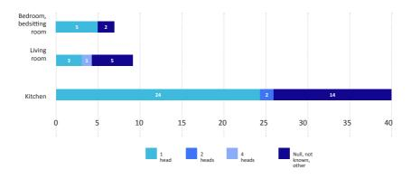
Figure 2. Number of sprinkler heads which activated by location with inside the flat
