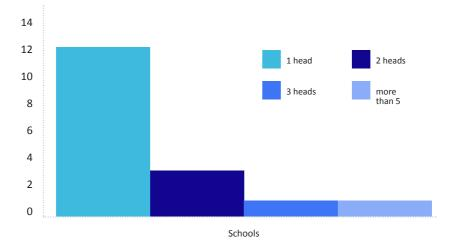
Figure 2: Number of sprinkler heads which operated
