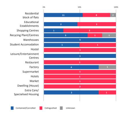
Figure 3 The effectiveness of the sprinkler system containing, controlling, or extinguishing the fire.
